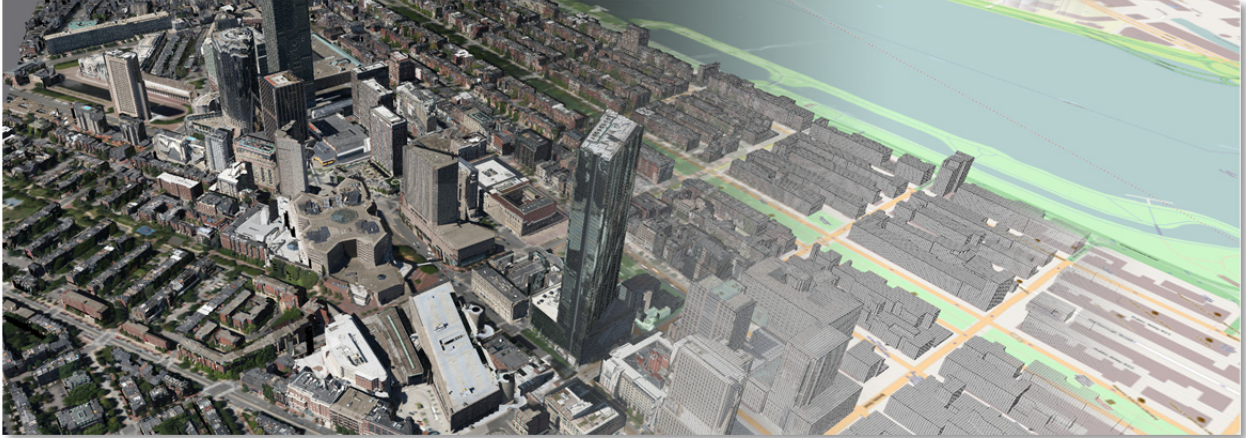
Figure 1. Urban Modeling. A complex urban area (left) is automatically obtained using volumetric reconstruction with surface graph cuts (middle) computed from aerial imagery and GIS-style parcel/building data (right). Our methodology uses photo-consistency to robustly recreate 2.5D building structures and surface graph cuts to assemble seamless and coherent textures despite occlusion, geometry, and calibration errors.
